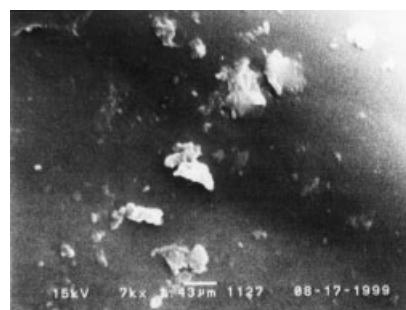
Figure 3 Scanning electron microscope a photograph showing the surface morphology of unreduced PVAc-AgNO 3 /PET (AgNO 3 30 wt%) a: A TOPCON SM-300 scanning electron microscope (SEM) was used to inspect the coating surface.
